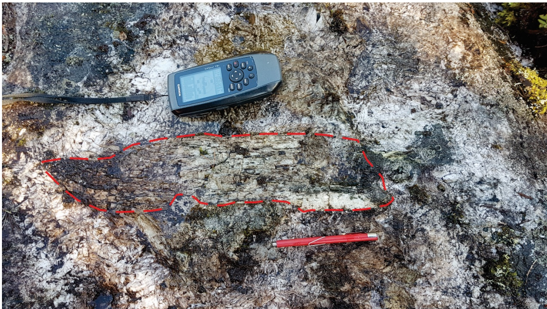
Figure 3 Pale green spodumene megacryst 30 cm long and 8 to 10 cm wide from Northeast Dyke – north outcrop.
