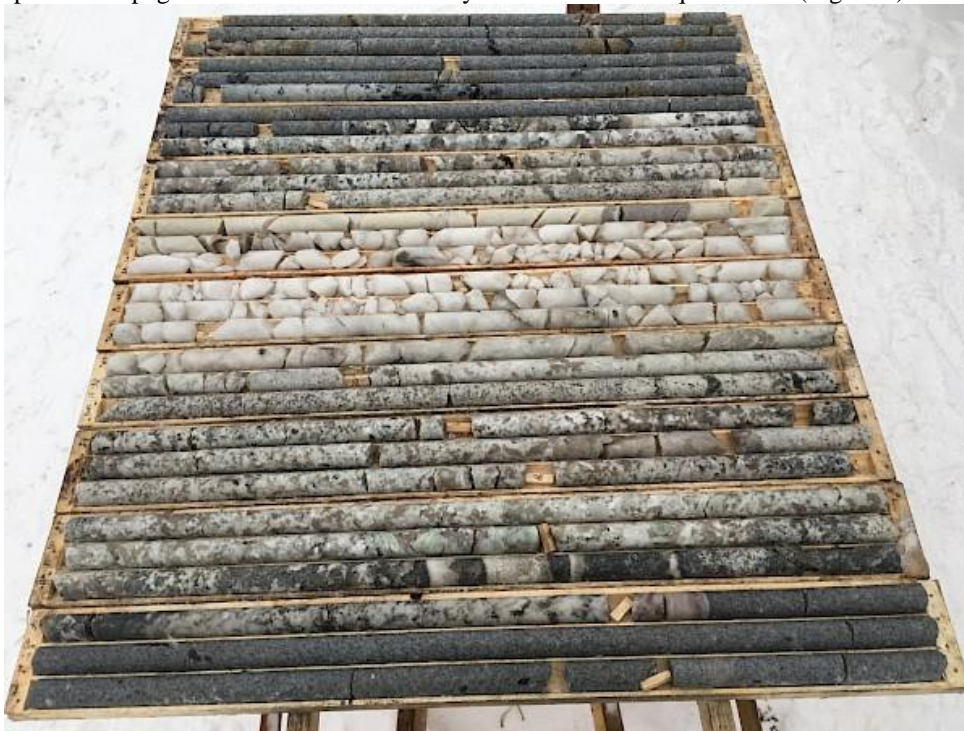
Figure 2 PWM-17-50 Main Dyke continuous pegmatite from 11.18 to 43.2 m. Note abundance of spodumene in boxes 3 and 4 and 7 to 9. Quartz core is in boxes 5 and 6.
