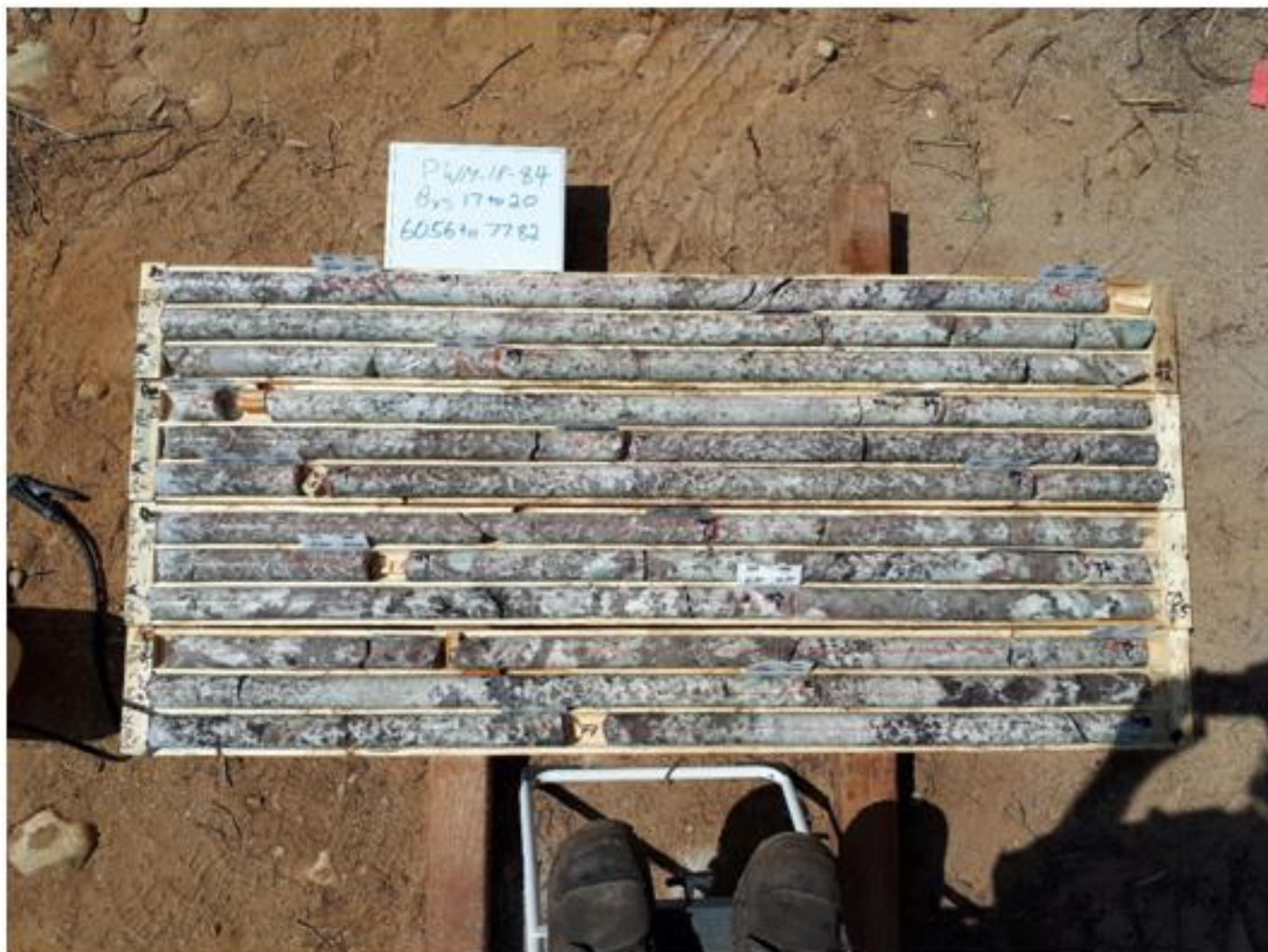
Figure 2 PWM-18-84, boxes 17 to 20, spodumene granite with up to 15% spodumene (boxes 17 to 19) and spodumene pegmatite with coarse-grained spodumene and up to 30% spodumene (boxes 19 and 20), Main Dyke, Case Lake.
