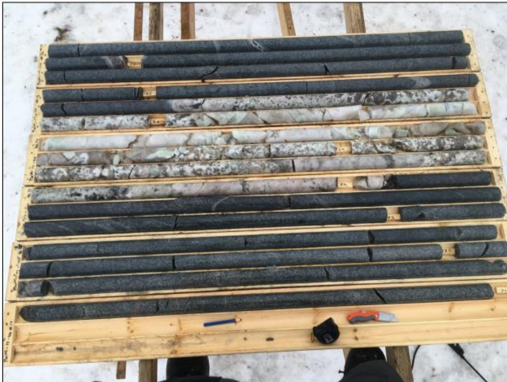
Figure 1 PWM-17-44, Boxes 12 to 17, photo of new spodumene pegmatite dyke below the Main Dyke. Note abundant pale green
