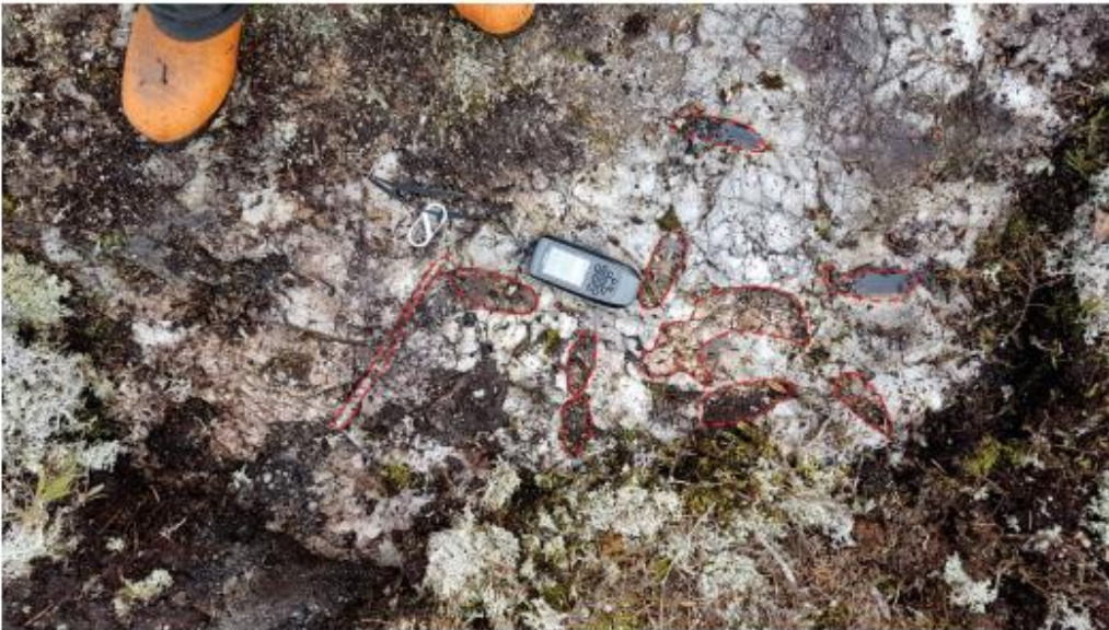
Figure 2 Oval cross sections of at least 8 beige spodumene megacrysts up to 14 cm across in quartz core of Northeast Dyke – south outcrop (sample 529461)
