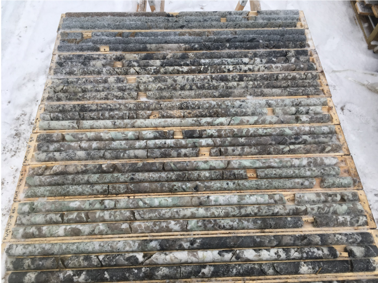
Figure 1 PWM-17-40 continuous pegmatite dyke from 8.23 to 45.93 m. Note the presence of high grade pale green spodumene in quartz core in boxes 5 to 8.
