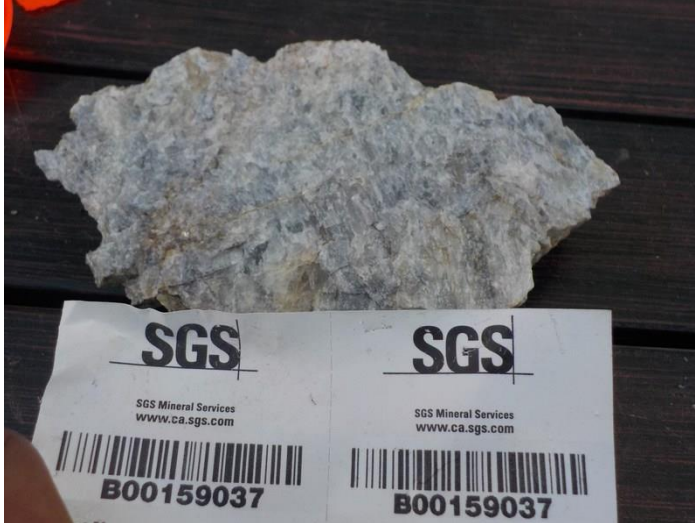
Figure 1 Grab sample 159037 of pure petalite with 4.43 % Li 2 O from Marko's pegmatite, Paterson Lake Property, Ontario. (CNW Group/POWER METALS CORP)
