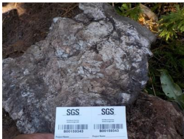
Figure 1 Sample 159343 with coarse-grained white petalite, 2.76 % \text{Li}_2\text{O} , Jesse's Pegmatite, Paterson Lake. (CNW Group/POWER METALS CORP)
