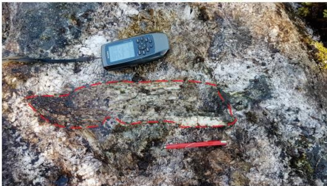
Figure 3 Pale green spodumene megacryst 30 cm long and 8 to 10 cm wide from Northeast Dyke – north outcrop (sample 529460)
