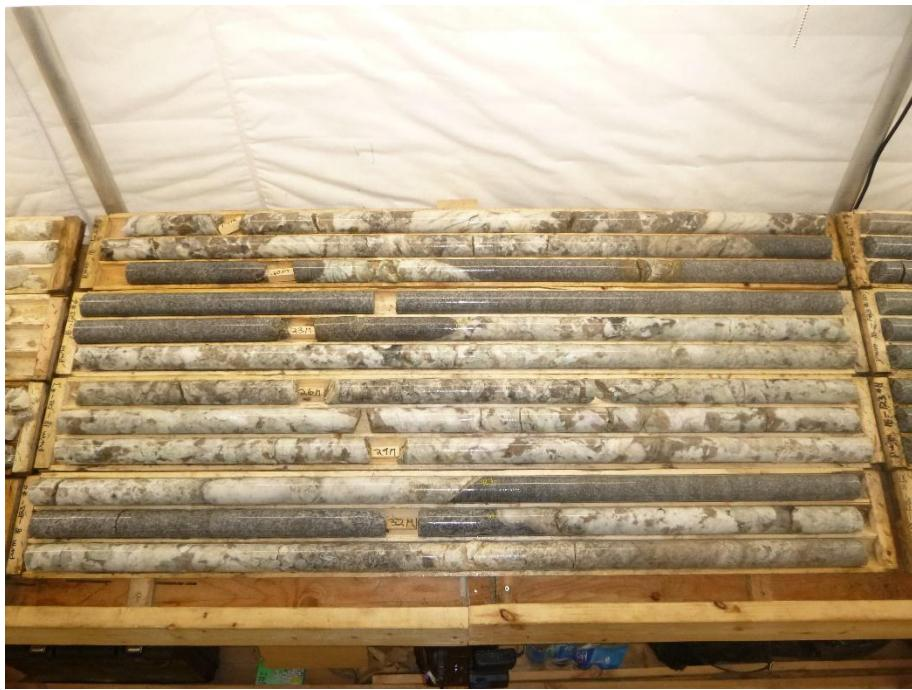
Figure 2 Spodumene pegmatite, PWM-18-123, boxes 5-8, 16.93-34.45 m, West Joe Dyke, Case Lake
