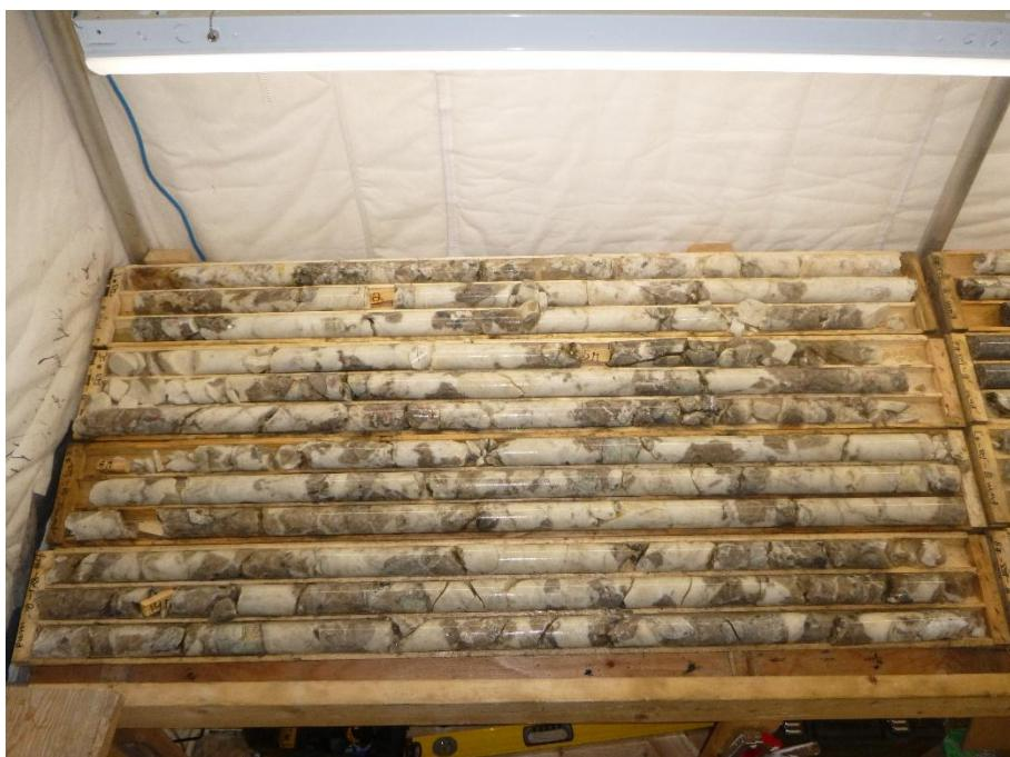
Figure 1 Spodumene pegmatite, PWM-18-123, boxes 1-4, 0.0-16.93 m, West Joe Dyke, Case Lake
